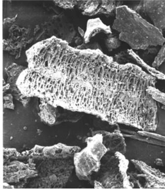
Figure 1. Suspension Burned RHA Porous Structure
